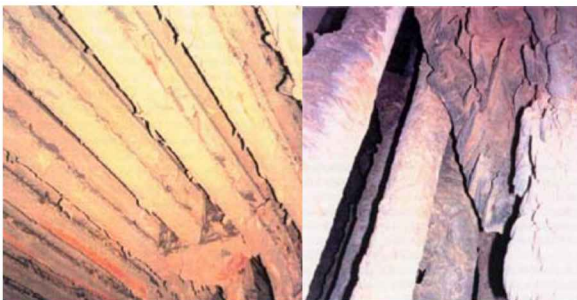
Figure 17: Pictures of deposits formed on superheater tubes of a steam boiler during waste wood combustion
